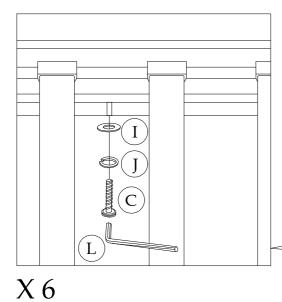
Check that the frame is central by adjusting the alignment of the frame and brackets before fully tightening all bolts. The metal frame should not contact the faux leather
