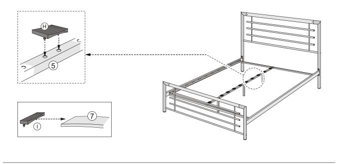
**Step 7**: Slide the slats (7) into hardware part (H) on the mid support (5) then push the ends into the side supports (3) firmly. *DO NOT use any power tools as this may damage the frame and will invalidate any claim.*
