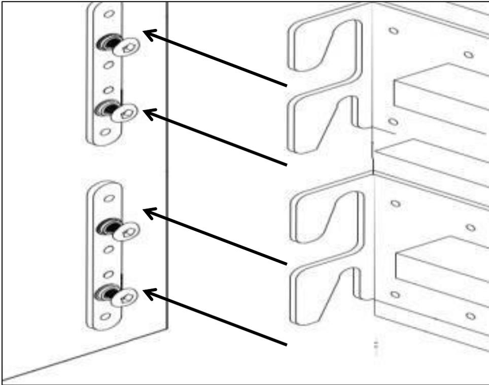
Slide the side rails onto the bolt of the Headend and use the Allan Key provided to tighten the bolts onto the brackets.
