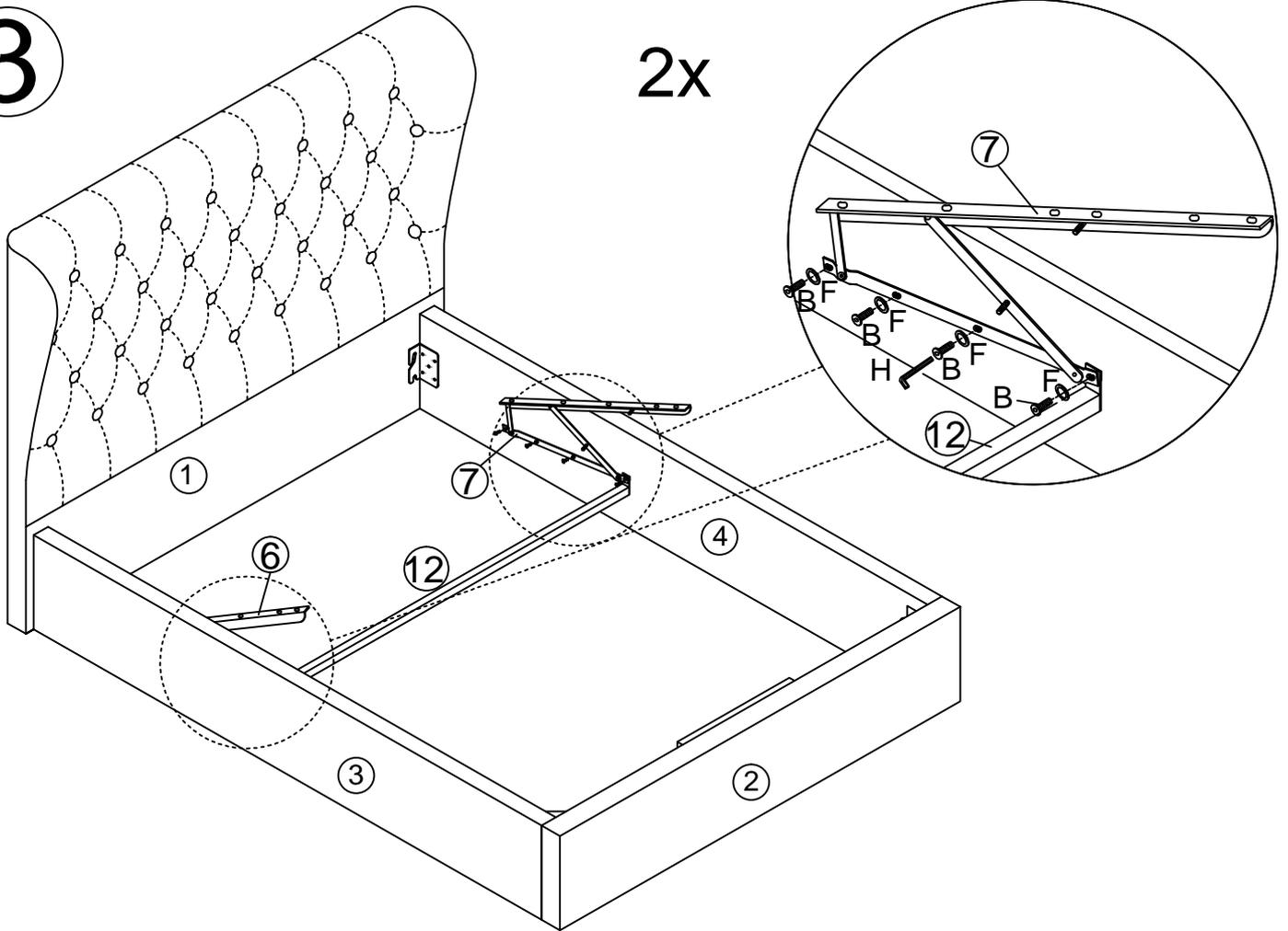
**ATTENTION:** The piston must be fitted wide end to the top as shown in the Assembly Instruction. Do not overtighten the nuts.
