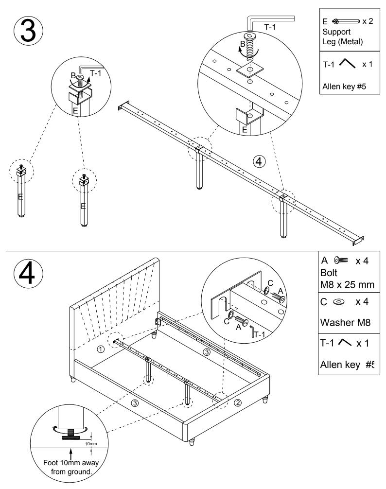
**ATTENTION:** After central rail and support legs being assembled, rotate adjustable feet to make support legs 10mm away from the floor. Support legs would touch the floor when a mattress is put on the base.
