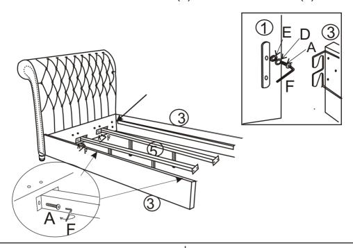
STEP 5 FIXING SIDE RAILS(3) TO FOOTBOARD(2) STEP 6 FIXING CENTRE SUPPORT BAR(5) TO FOOTBOARD(2)
