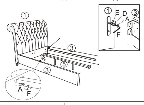
STEP 5 FIXING SIDE RAILS(3) TO FOOTBOARD(2) STEP 6 FIXING CENTRE SUPPORT BAR(5) TO FOOTBOARD(2)
