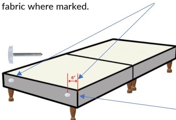
If the holes are not marked, they are located 6" from the edge of the base
