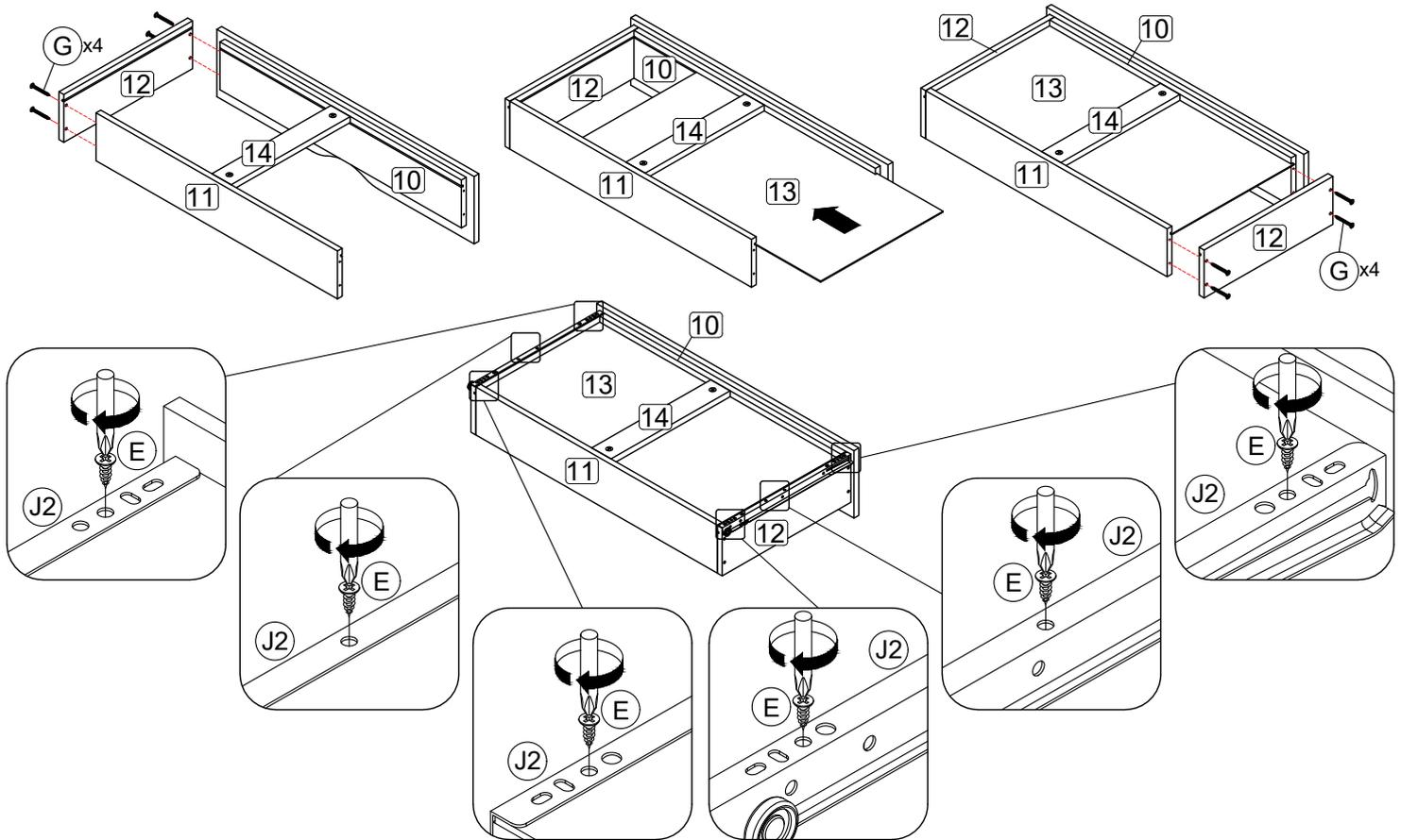
**Step 10:** Assemble the drawer in place along the drawer slides.
