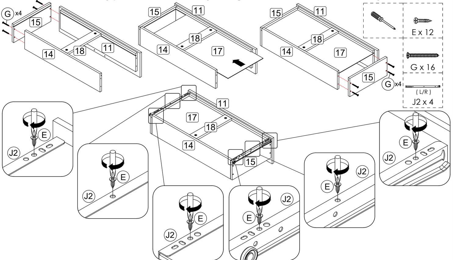
**Step 11:** Assemble the drawer components using hardware E, G and J2.
