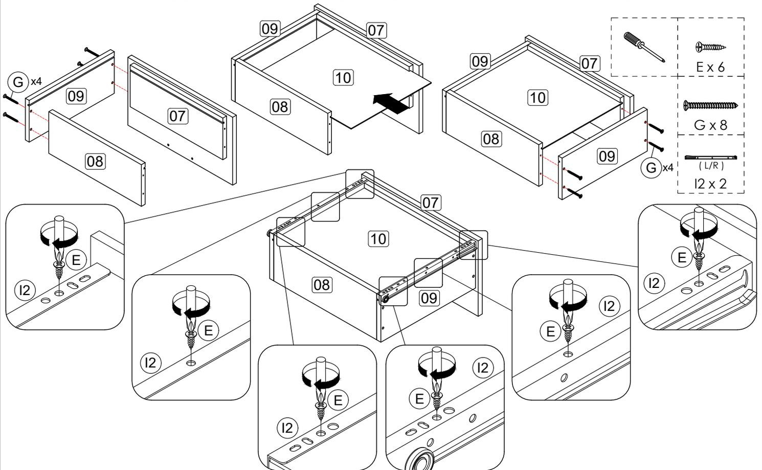
**Step 8:** Assemble the drawer in place along the drawer slides.
