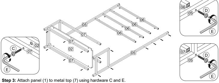
: Attach panel (1) to metal top (7) using hardware C and E.
