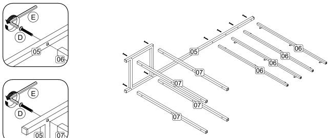
Step 2: Attach metal top (6) and metal bottom (7) to metal frame side (5) using hardware D and E. Attach panel (2) to metal bottom (7) using hardware C and E. DO NOT use any power tools as this may damage the frame and will invalidate any claim.
