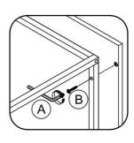
Step 4: Attach the Small Metal Top (7) to Small Top panel (5) using hardware A and B.
