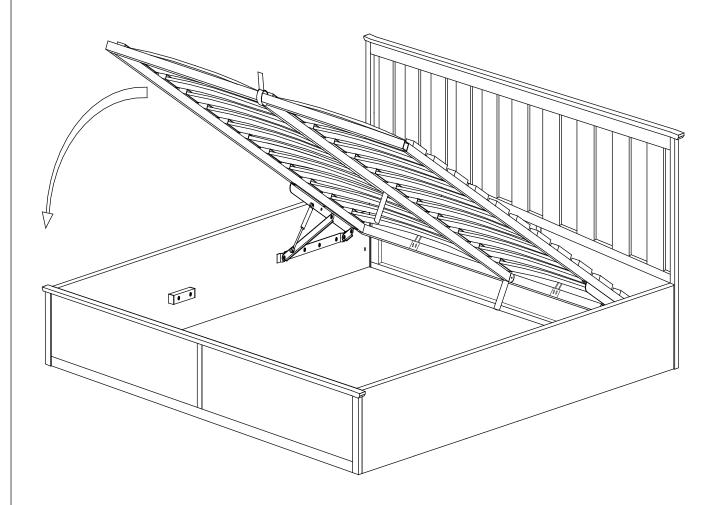
Lift with the strap (H12) and close with the strap. The strap should always be accessible. Take care not to lean over the bed when lifting, if the mattress is thin and light, the frame may rise quickly. The speed of closing will also depend on the weight of the mattress so always keep fingers well clear of the metal frame.
