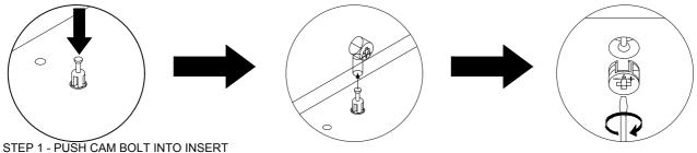
STEP 2 - ALIGN THE CAM BOLT WITH THE HOLE AND PUSH TOGETHER UNTIL FLUSH. ( MAKE SURE THE ARROW OF THE CAM LOCK IS POINTING TOWARD ON THE EDGE OF THE PANEL.)
