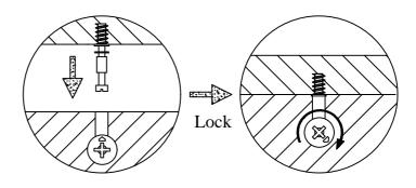
Use a flat blade screwdriver to tighten the cam nuts. A quarter turn clockwise is all that is needed.
