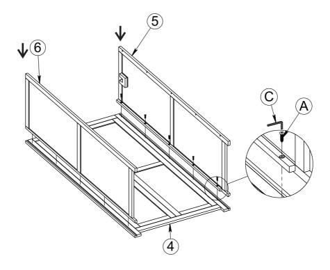
Note: All screws must install according to the working hole.
