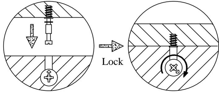
Use a flat blade screwdriver to tighten the cam nuts. A quarter turn clockwise is all that is needed.
