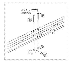
Do not fully tighten the screw yet until Step 7
