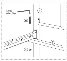
Do not fully tighten the screw yet until Step 7
