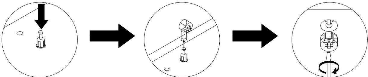
STEP 1 - PUSH CAM BOLT INTO INSERT
