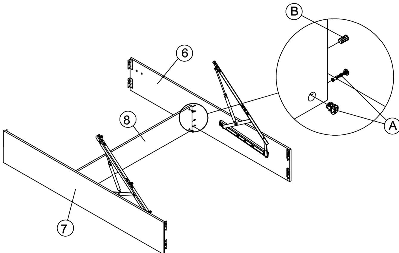
Step 6: Fix side rail to the headboard and footboard with hardware as shown.
