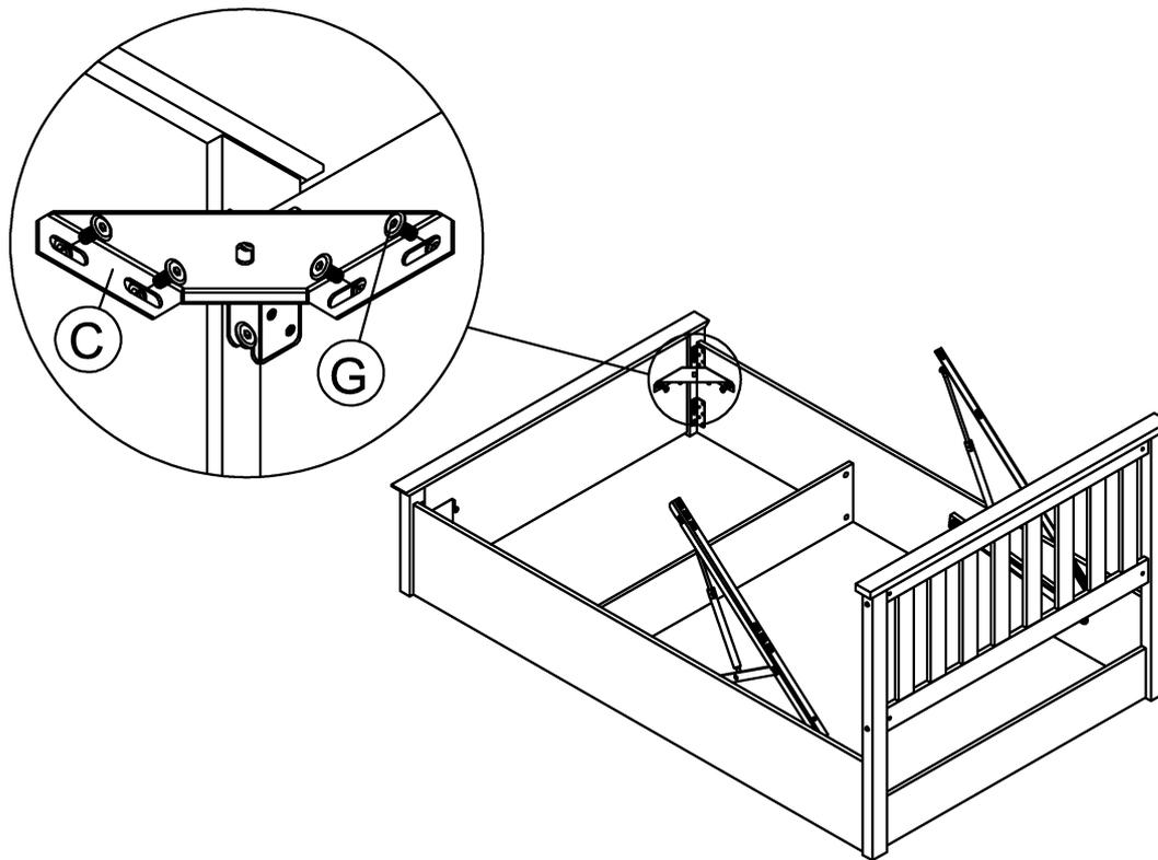
Step 8: Join together all the bed base parts (11),(12),(13),(14) and (15) using hardware parts G,X & R and also slide part P onto Part 14 before bolting together. And then attach hardware parts J as shown. Important
