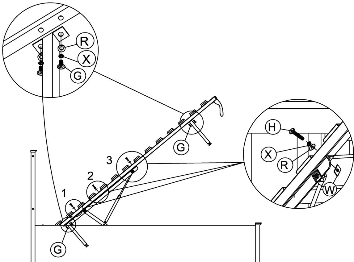
Step 11: Adjust the bed base making sure that the distance to the footboard is approximately **15 mm** to above. Tighten all bolts and screws now.
