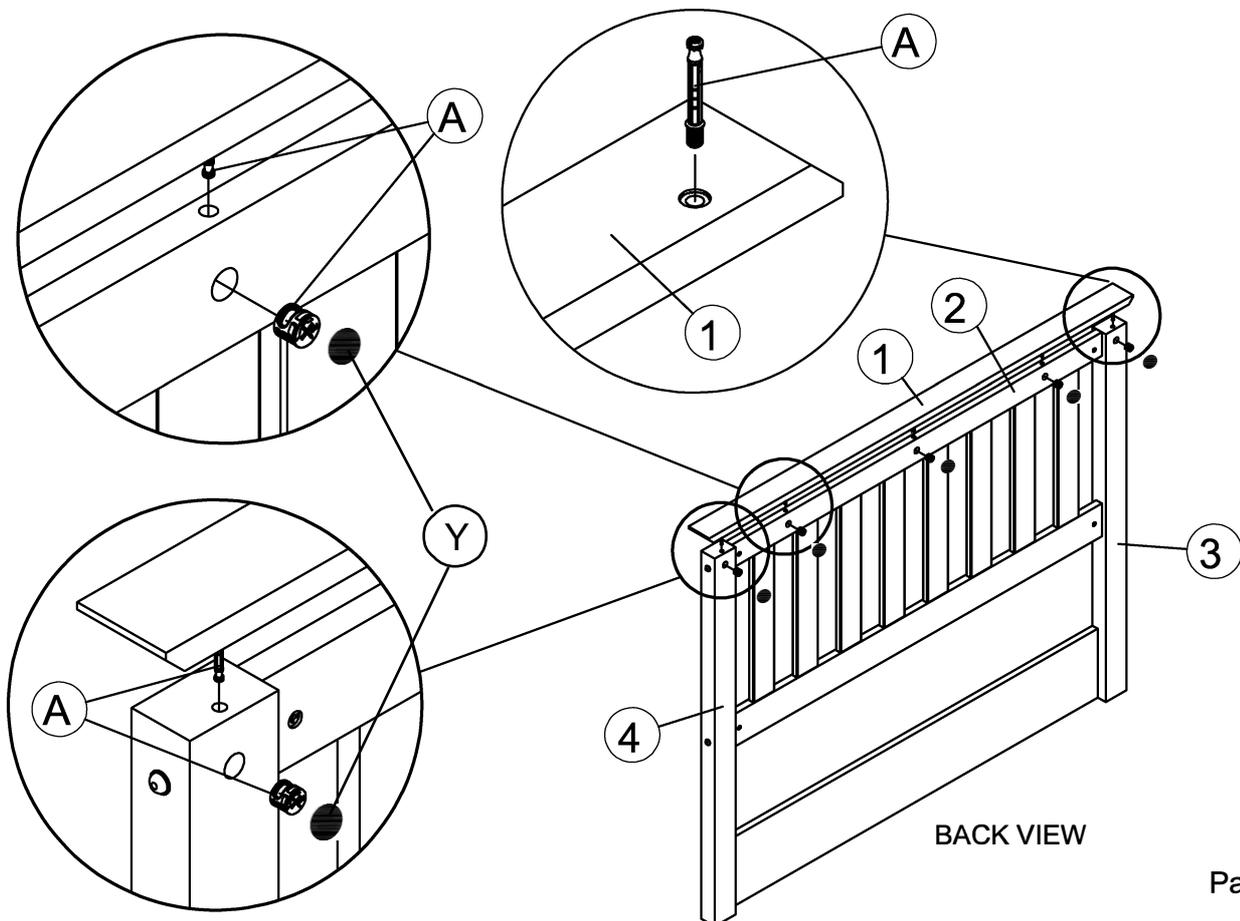
Step 3: Firstly screw the minifitpart A to the top bar (1) as shown and then fix the top bar (1) to the footboardframe (5) using hardware parts A; then paste the sticker Y.
