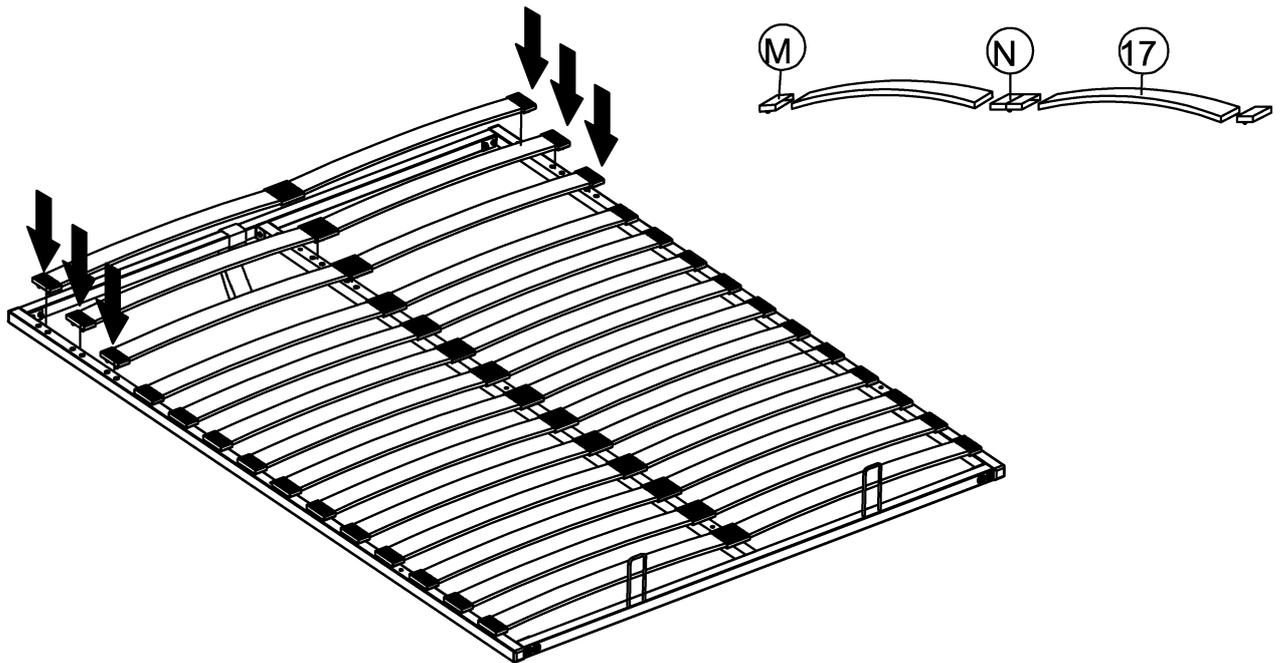
Step 10: Assemble the bed base on the right & left hydraulic frame and fix bolts L starting from ' 1 ' to ' 3 ' as shown and fix the support leg (16) to the bed base as shown.
