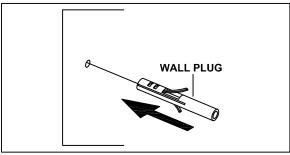
STEP 3: Pull the screw in the wall plug hole
