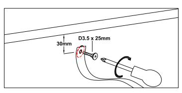
STEP 2: Make a hole on the wall and pull the wall plug in
