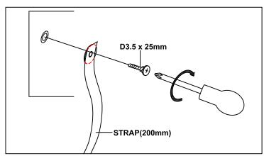
NOTE: Wall fixing are not supplied with this product as different wall materials require different types of fixing devices (such as Rawl plugs on brick work). You must use fixing devices suitable for the type of wall you intend to mount this product to. Please ensure that the head of any screw used has a diameter greater that the diameter of the mounting hole on the product and that the fixing is safe and secure before use.
