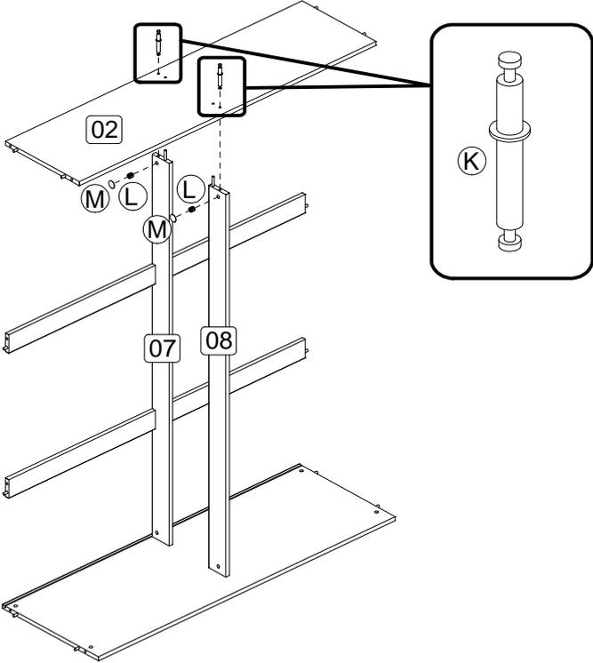
**Step 5:** Attach the self divider (6) and the top panel (1) using hardware parts L and M with a screwdriver (not provided).
