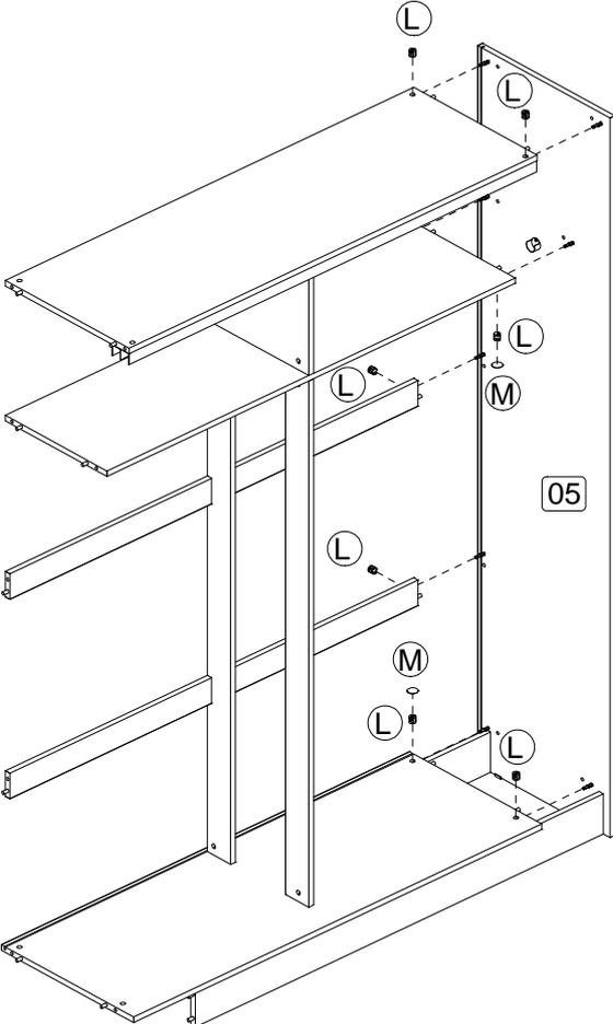
**Step 8:** Position the hanging rail R4 then attach the left panel (4) using hardware parts L and M with a screwdriver (not provided)
