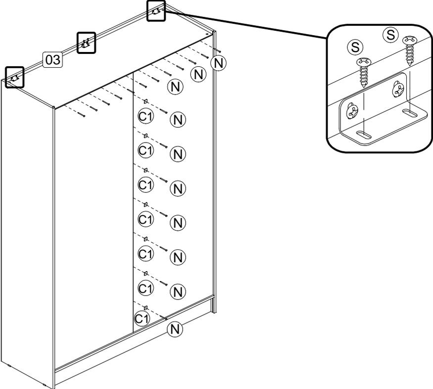
**Step 11:** Attach the doors (11) and (12) as shown in the diagram.
