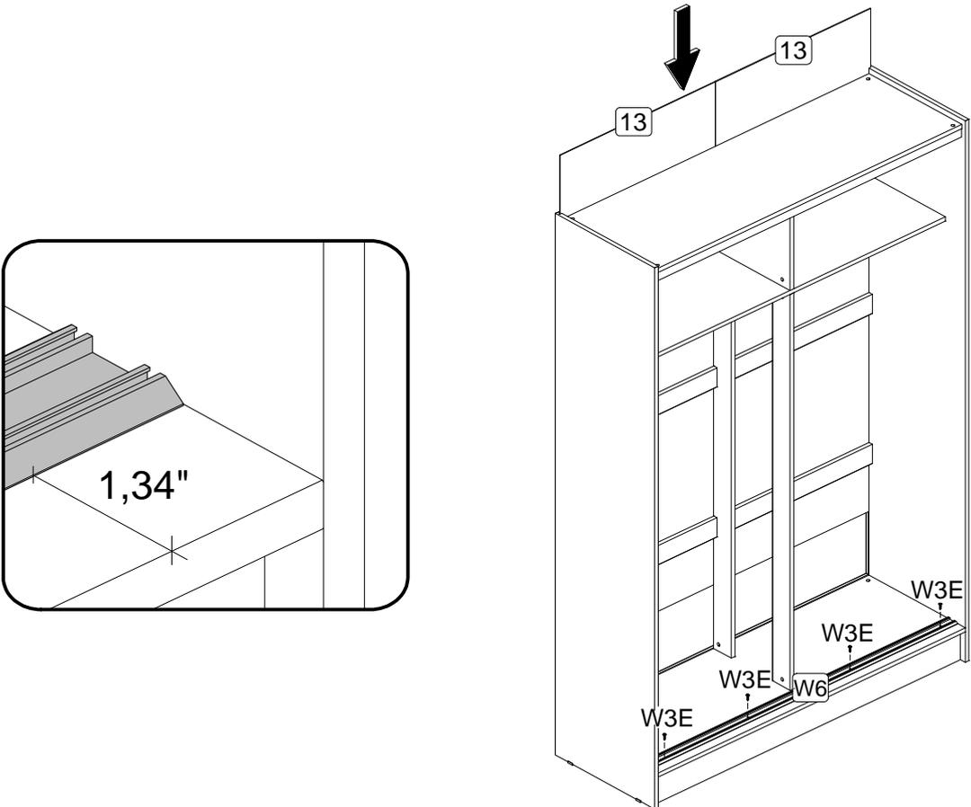
**Step 10:** Secure the back panels (13) using hardware parts C1 and N with a small mallet (not provided). Attach the top plinth (3) using hardware part S with screwdriver (not provided).
