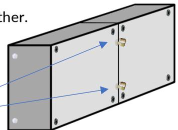
**With the side and front opening divan bases**, place the u-clips onto the top rails where the 2 halves meet.
