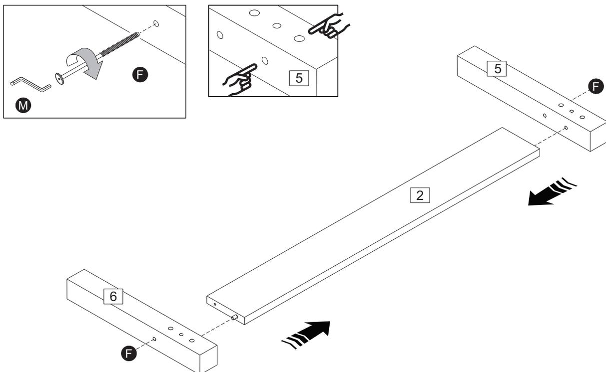
**Step 8:** Attach the side rails to the headend posts at the same time using hardware parts G, H and M. **Vendor:** S000238
