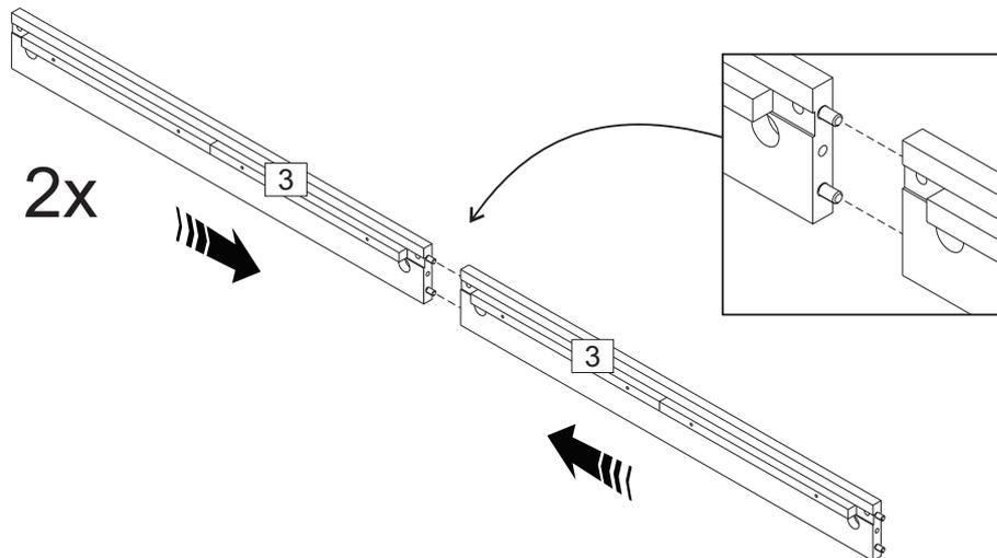
**Step 3:** Join the two rails (3) and attach the support leg (8) using hardware E, J, K (spanner not provided).
