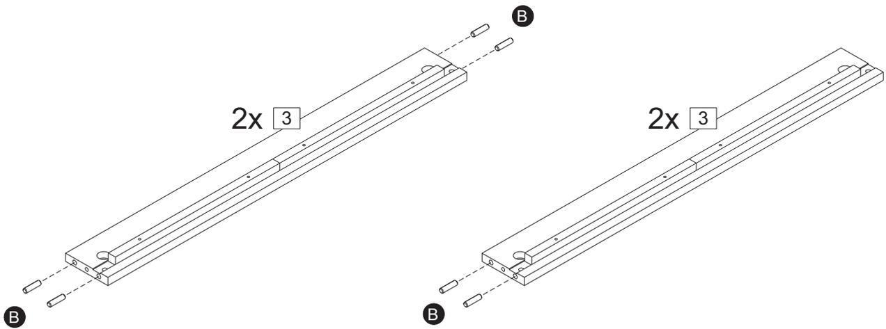
**Step 2:** Insert the dowels B into both siderails as per the drawing.
