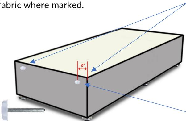
If the holes are not marked, they are located 6" from the edge of the base
