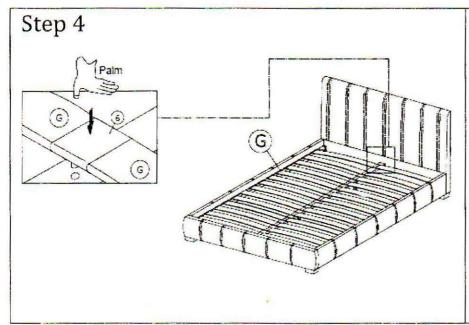
4.1 Slot the first slat (G) into the centre slat cap (6) and insert a second slat (G) into the centre slat cap (6) on the opposite side. Attach an end slat cap (5) to the second slat before pressing the caps into the corresponding holes on the centre rail (D) and side rail (C).
