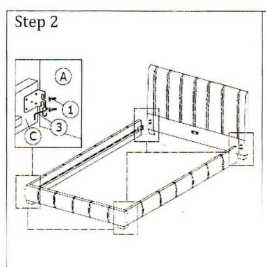
2.1. Attach the side rails (C) to the headboard (A) & footboard (B) with M8 x 30mm screws (1).
