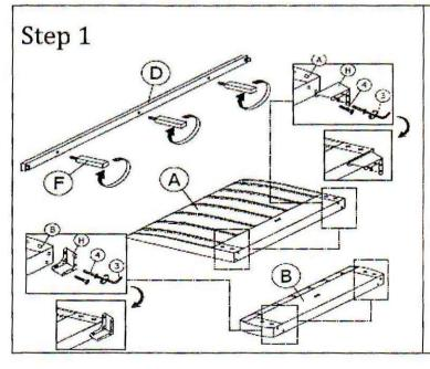
1.1 Attach the corner feet (H) to the headboard (A) & footboard (B) with the M8 x 20mm screws (4).
