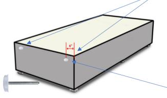
If the holes are not marked, they are located 6" from the edge of the base
