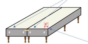
If the holes are not marked, they are located 6" from the edge of the base
