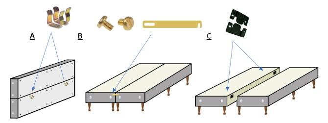
• Insert the headboard bolts into the locator holes at the headend of the base by piercing the fabric where marked.
