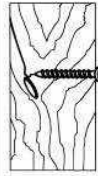
Wood If fixing to wood make sure that it isn't chipboard as screws can easily pull away from the core structure
