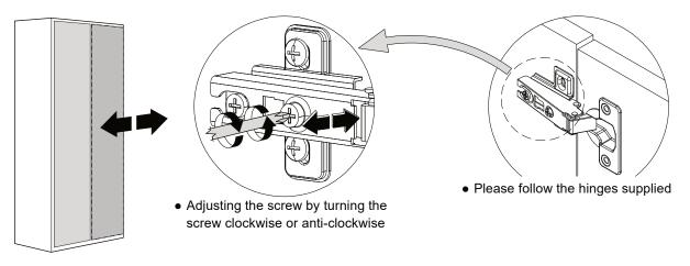
B. Vertical adjustment (Moving door up-down) via the slot on the mounting plate
