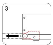
• Ensure the roller is in the track of drawer slide before push to the end.
