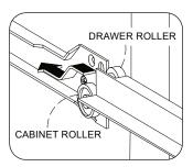
Locate both roller on drawer box and roller on cabinet.
