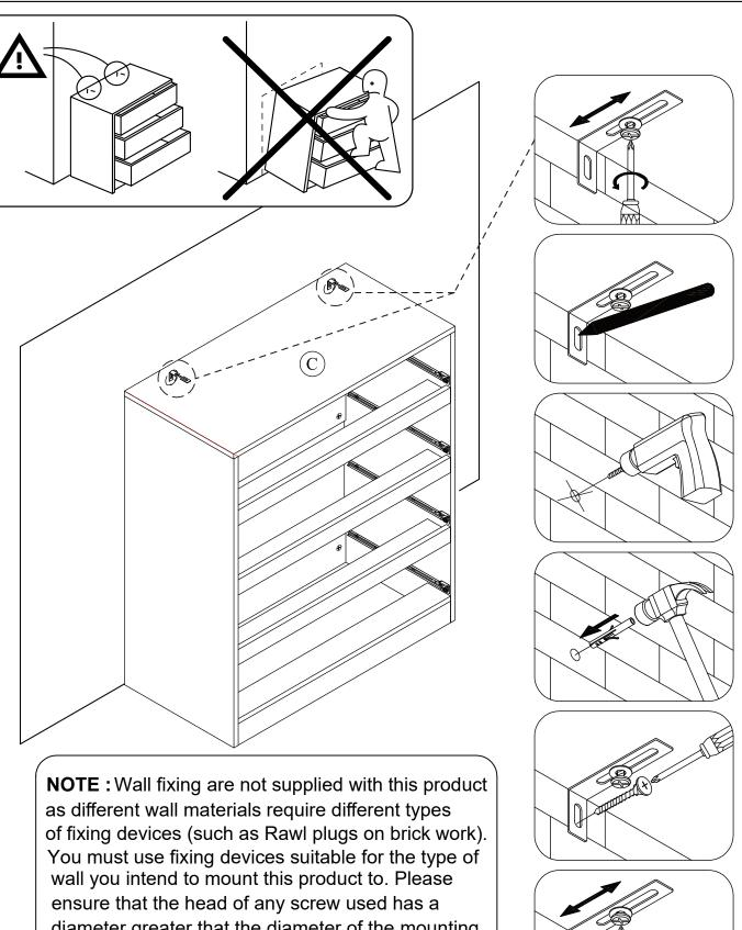
diameter greater that the diameter of the mounting hole on the product and that the fixing is safe and secure before use.
