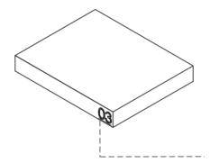
USE ALCOHOLIC CLEANING SOLUTION ONLY TO REMOVE PART NUMBERS
