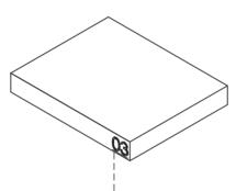
USE ALCOHOLIC CLEANING SOLUTION ONLY TO REMOVE PART NUMBERS
