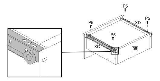
Step 11: Insert the drawers on the metallic slide as shown bellow.
