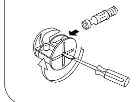
The head of the cam bolt goes into the open mouth of the cam nut. You then turn the cam nut so it tightens over the bolt.
