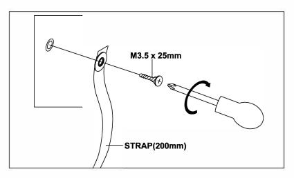
NOTE: Wall fixing are not supplied with this product as different wall materials require different types of fixing devices (such as Raw plugs on brick walls). You must use fixing devices suitable for the type of wall you intend to mount this product to. Please ensure that the head of any screw used has a diameter greater than the diameter of the mounting hole on the product and that the fixing is safe and secure before use.
