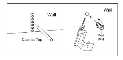
STEP 3: Pull the screw in the wall plug hole
