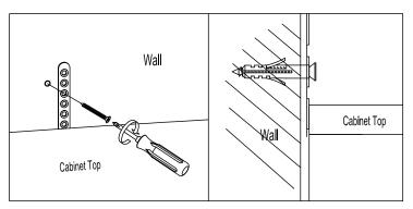
**NOTE:** Wall fixings are not supplied with this product as different wall materials require different types of fixing devices (such as Rawl plugs on brick work). You must use fixing devices suitable for the type of wall you intend to mount this product to. Please ensure that the head of any screw used has a diameter greater that the diameter of the mounting hole on the product and that the fixing is safe and secure before use.
