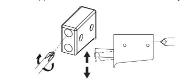
VII When unit is level, tighten lower screws clockwise so clamping unit to wall - do not over-tighten.
