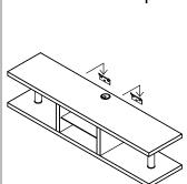
VI Hang the cabinet onto the brackets by carefully aligning the end panels so they just miss the outer sides of the brackets. To make cabinet level, turn upper screw clockwise on one side only.
