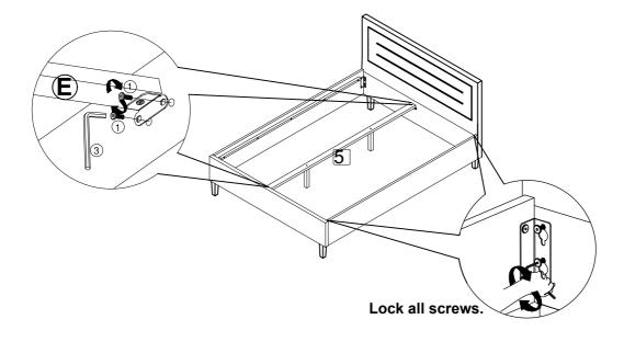
Step 5: Affix the slat (D) to the side rail support wood. Tighten all the self tapping screws(4).
