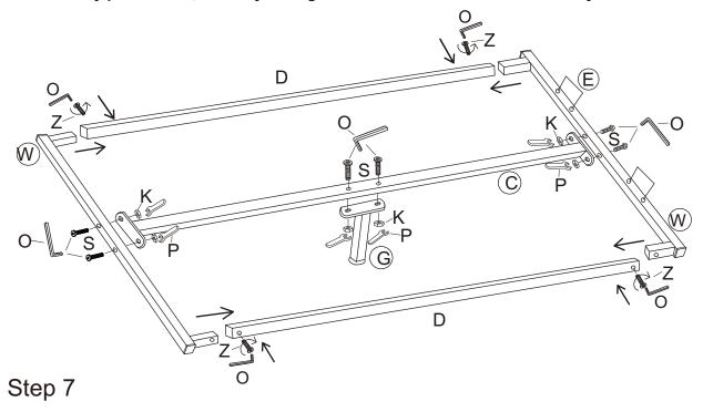
To attach the metal frame(W/C/D) and cross support bar(X)to the gas lift pre-fixed to the side rails, you will need to use hardware parts 4X M8x65mm Bolts(A1) , 2 XM8x45mm Bolts(L) and 6x Nuts (K) with the M5 allen key(O) and the spanner(P).
