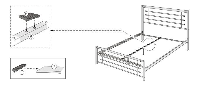
**Step 7**: Slide the slats (7) into hardware part (H) on the mid support (5) then push the ends into the side supports (3) firmly. **DO NOT use any power tools as this may damage the frame and will invalidate any claim.**
