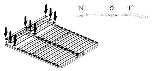
**Step 8**: Insert the small base panel (9) and large base panels (10). DO NOT use any power tools as this may damage the frame and will invalidate any claim.
