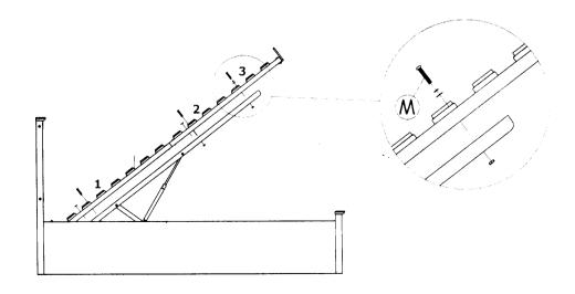
**Step 10**: Adjust the bed base making sure that the distance to the footboard is approximately 10 - 15 mm. Tighten all bolts and screws now.
