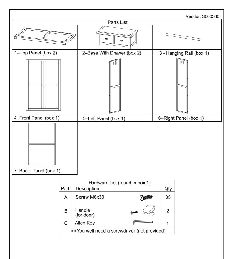
Note: All screws must install according to the working hole. Step 1: Attach the left panel (5) and right panel (6) to the front panel (4) using hardware parts A and C. DO NOT use any power tools as this may damage the frame and will invalidate any claim.
