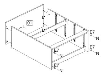
**Step 6:** Connect the back panels (10) using the spine (A6) and secure using hardware part N and a small mallet (not provided).
