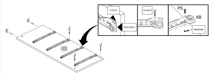
**Step 2:** Attach the metallic slide (XA) to the left panel (2) using hadware part P5. Insert hardware part E using a small mallet (not provided) and the part J using screwdriver (not provided).
