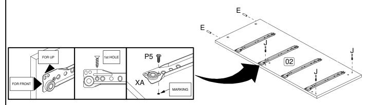
**Step 3:** Insert hardware parts E and J as shown using hardware part A1, a small mallet and a screwdriver (not provided).
