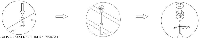
STEP 1 - PUSH CAM BOLT INTO INSERT
