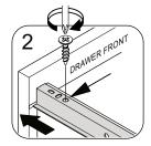
• Fix the first screw on the third hole from front.
