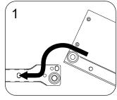
• Align the roller on drawer box on top of the roller on cabinet.
